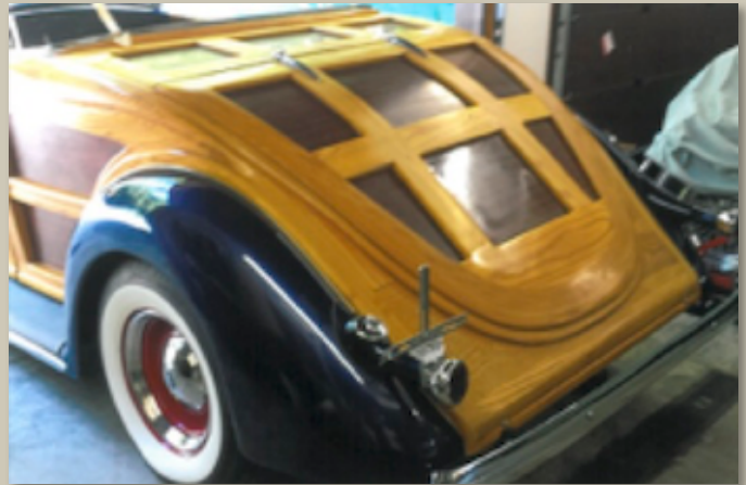
#12 I tried to put all the curves in the body that's on a '36 roadster, but instead of the little rumble seat, I put a large trunk like a 40 Ford coupe. The spare tire mounted on the trailer hitch, but looks stock.
